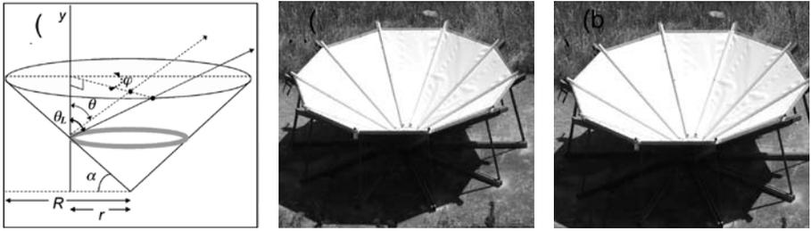
**Figure 1** Integration scheme for the funnel shape ( $0 < \theta < \theta_L$ ,  $0 < \phi < 360^\circ$  and  $0 < r < R$ ). (b) Photo of the funnel-shaped condenser ( $7.3 \text{ m}^2$  surface area with  $60^\circ$  cone angle,  $30^\circ$  from horizontal). The internal surface of the experimental condenser is coated with OPUR ([www.opur.fr](http://www.opur.fr)) low density polyethylene film insulated from below with 3cm styrofoam.
