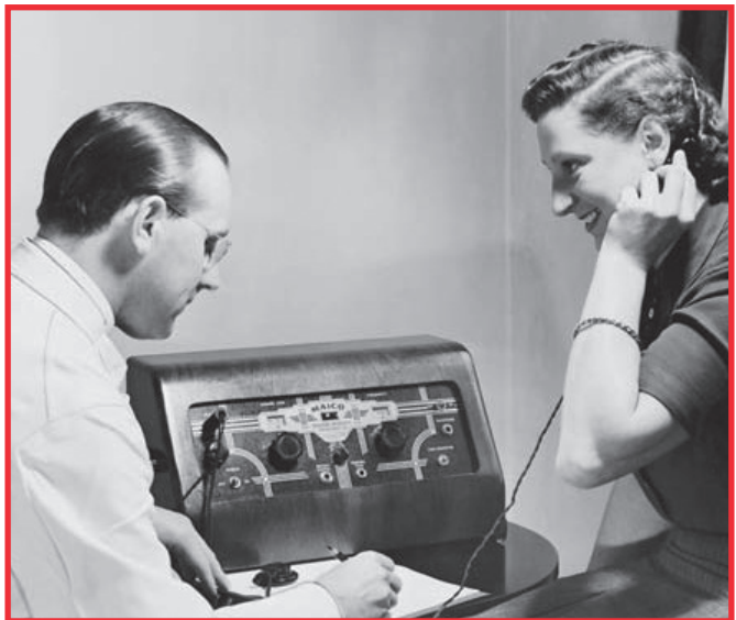
Fig. 10: Oticon hearing test conducted with audiometer, the late 1930s. Picture derived from Oticon (2004)
