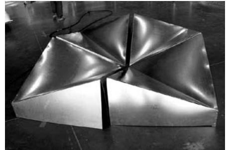
Figure 5 Inverted pyramid with an angle 30^\circ from horizontal and four condensation side. The section at the top is 1 m x 1 m.
