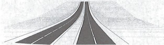
Transition of a 2% downgrade to a 3% upgrade effected by a liberal curve 3,000 feet long, vertical radius about 60,000 feet.
