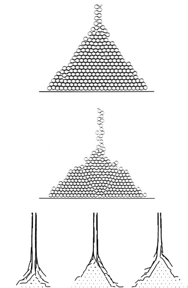
Figure 1: The five main pertinent spatial figures of 'the Spatial Dynamic Dune Effect' we obtained: (1) piling, (2) internal heterogeneous constraints, (3) surface avalanches, (4) internal collapses, (5) auto-similar sub-pilings.
